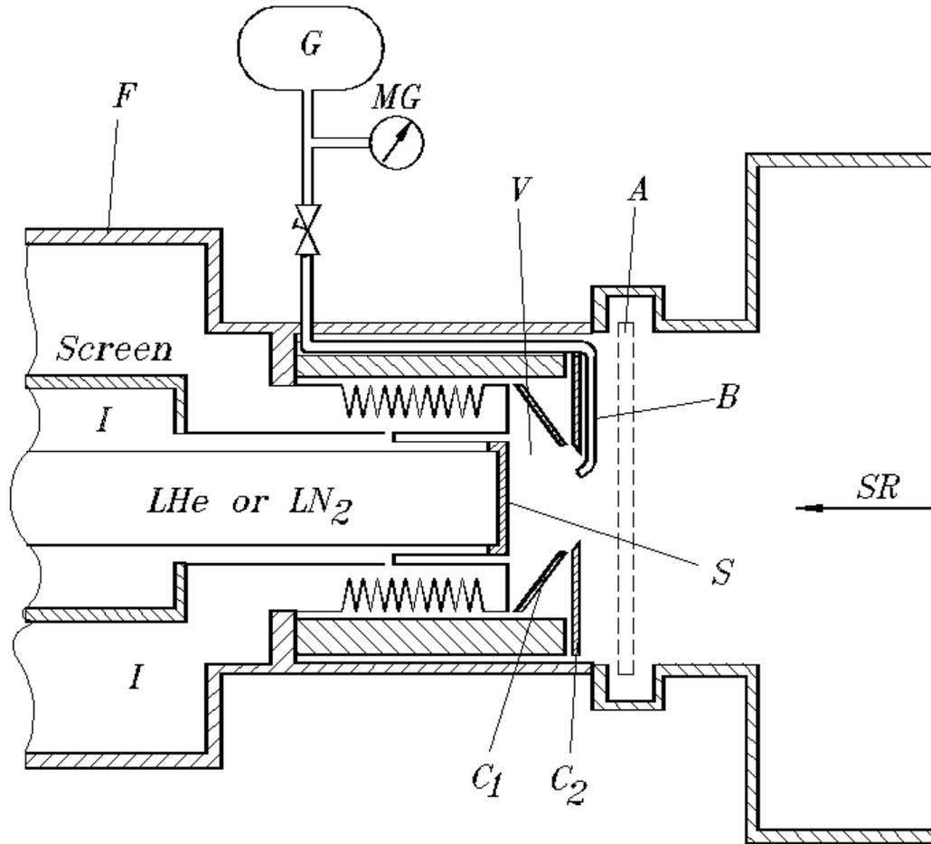
Figure 1. The experimental set-up on the synchrotron radiation beam line. *F* is the cryostat, *I* is the isolating vacuum, *V* is the experimental volume which can be separated from the beam line with the valve *A* shown in the closed position. The membrane gauge *MG* measures the gas pressure in the volume *G* which is injected via the pipe *B* and condensed onto the substrate *S* at cryogenic temperature. *C*<sub>1</sub> and *C*<sub>2</sub> are the insulated collector electrodes.
