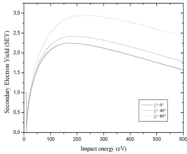
Fig. 1 Secondary Electron Yield for copper with three different impact angles
