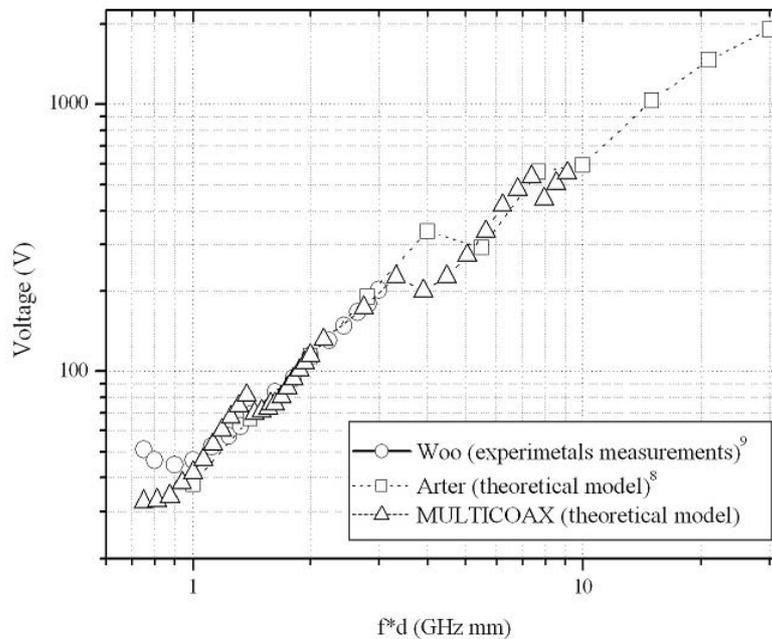
Fig. 6 Comparison between experimental measurements [9] and an theoretical model [8].  $b/a=2.3$ ,  $Z= 50 \Omega$
