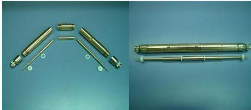
Fig. 2 Coaxial samples designed and measured at ESA/ESTEC laboratories
