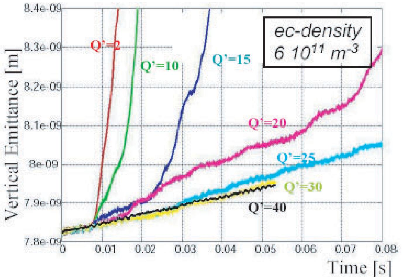
Emittance growth vs. time (for parametres of LHC @ injection)
