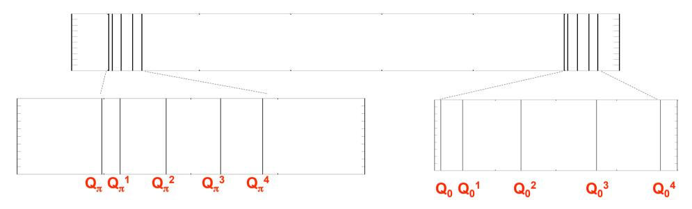
Due to the LR interaction all bunches are coupled as a result the  $\sigma$  and  $\pi$  modes split with sidebands with direction opposite with respect to the HO bb tune shift
