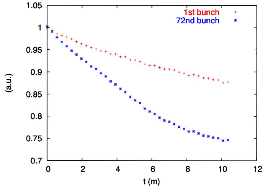
Comparison between the **bunch rms-length** (inferred by Gaussian interpolation of the shape signal) and **population** (inferred by summing up the channels of the shape signal) evolution along the coast of a bunch at the head of the train and at its tail.
