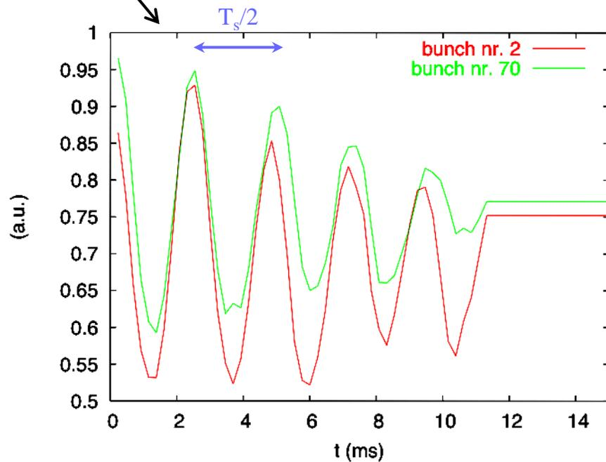
In the first supercycle the bunches were strongly mismatched in their buckets and performed damped quadrupole oscillations
