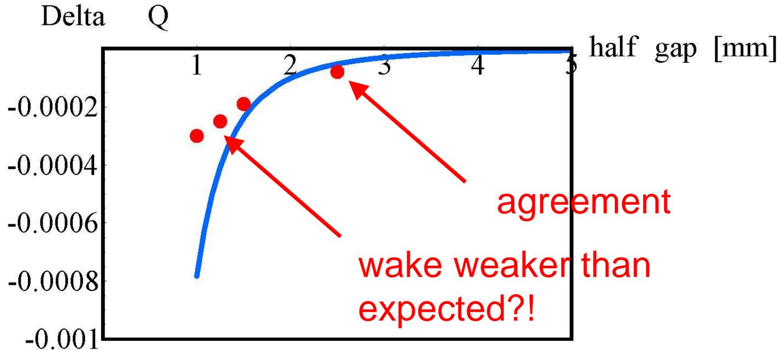
Expected tune shift of a pencil beam of constant intensity of  $8.5 \times 10^{10}$  protons, on which the measured data (from Marek Glasier's APC talk) are superimposed.
