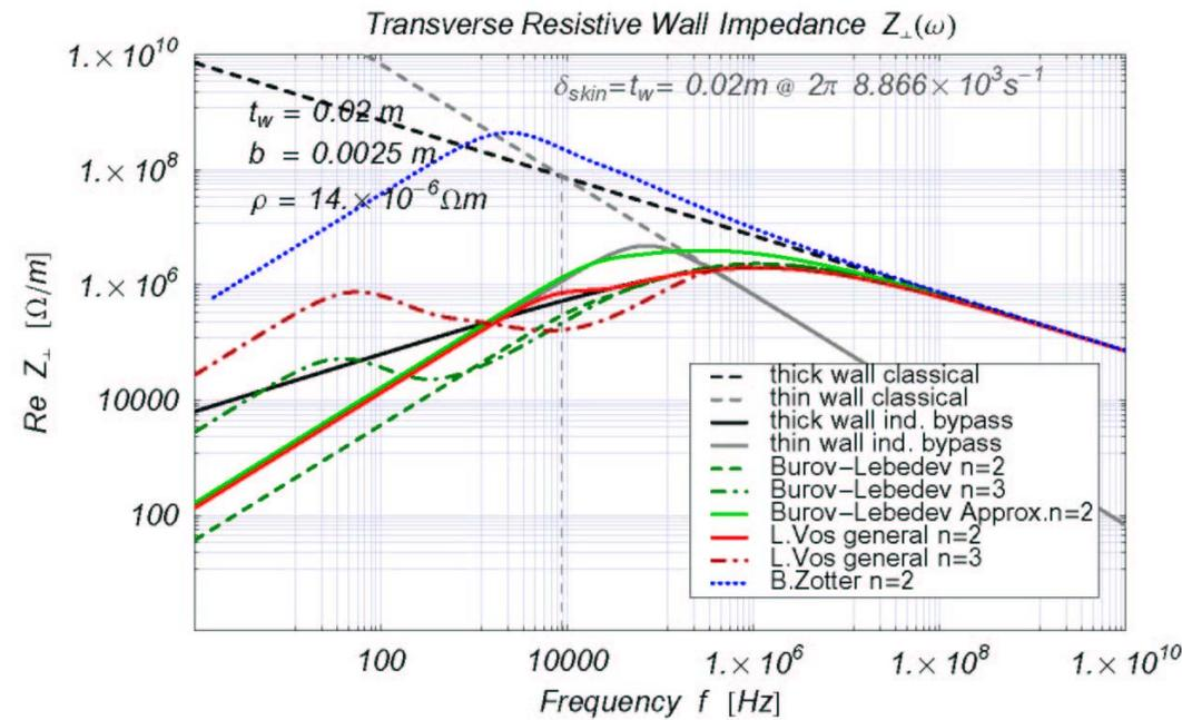
Predictions for the collimator impedance from calculations and formulae by various authors (compiled & plotted by A. Koschik).
