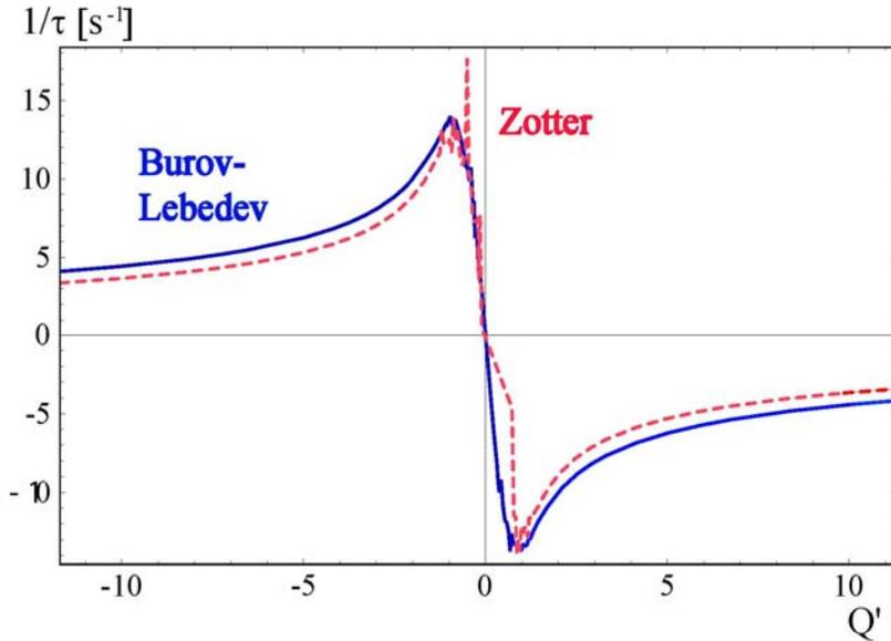
single-bunch vertical head-tail growth rates due to the collimator
