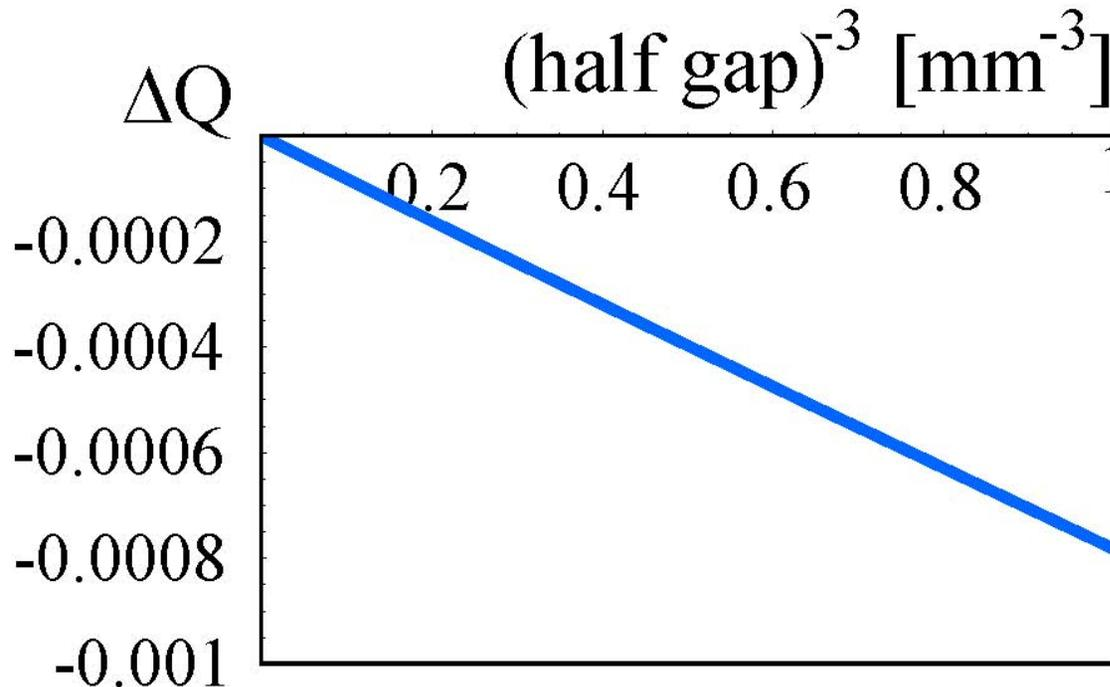
Expected tune shift for the SPS collimator experiment as a function of the inverse third power of the collimator half gap. The dependence  $\sim 1/b^3$  differs from observed dependence  $\sim 1/b$
