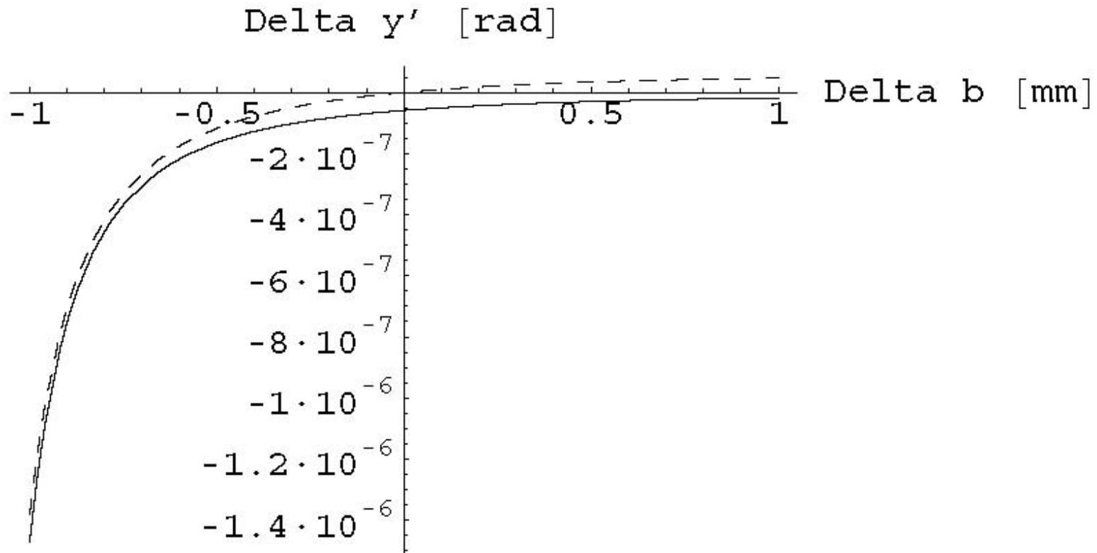
Collimator kick versus jaw position on one side: initial beam-jaw distance is 1.25 mm; the jaw on one side is then moved by 'Delta b'; either the opposite jaw is held fixed at a distance 1.25 mm (dotted), or it is kept at an infinite distance (solid).
