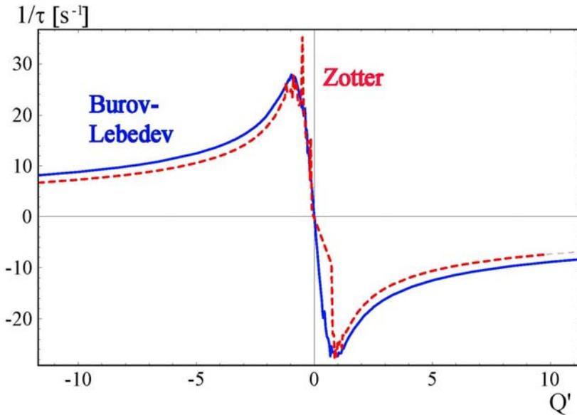
single-bunch horizontal head-tail growth rates due to the collimator
