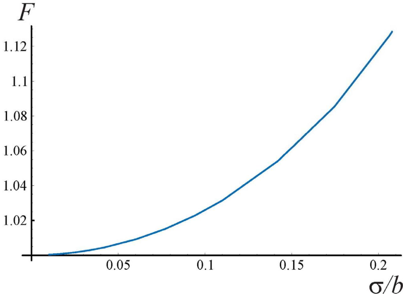
Piwinski form factor  $F$  for  $y/b \ll 1$  vs. the relative beam size
