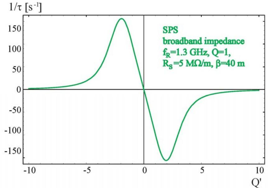
single-bunch horizontal head-tail growth rates due to the SPS horizontal broadband impedance.
