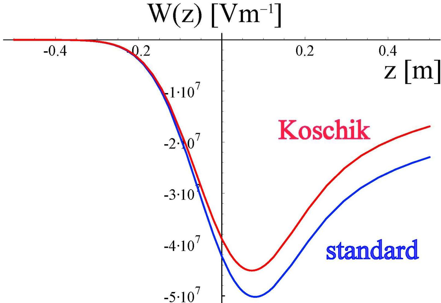
short-range resistive-wall wake field, obtained by folding the Green function wake with the bunch profile, for the SPS collimator computed from standard expression and using Koschik's formula
