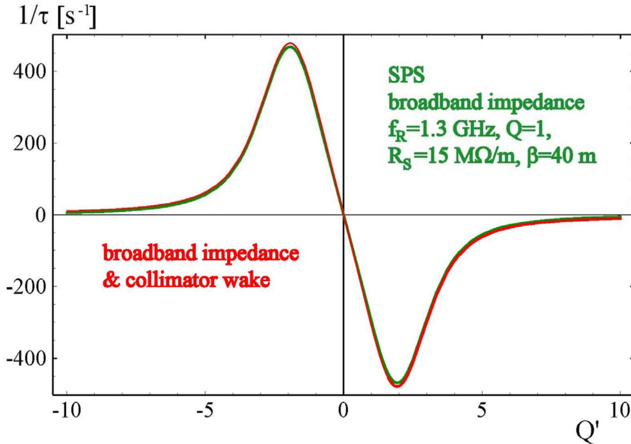
single-bunch vertical head-tail growth rates due to the SPS horizontal broadband impedance and with the additional effect of the collimator impedance.
