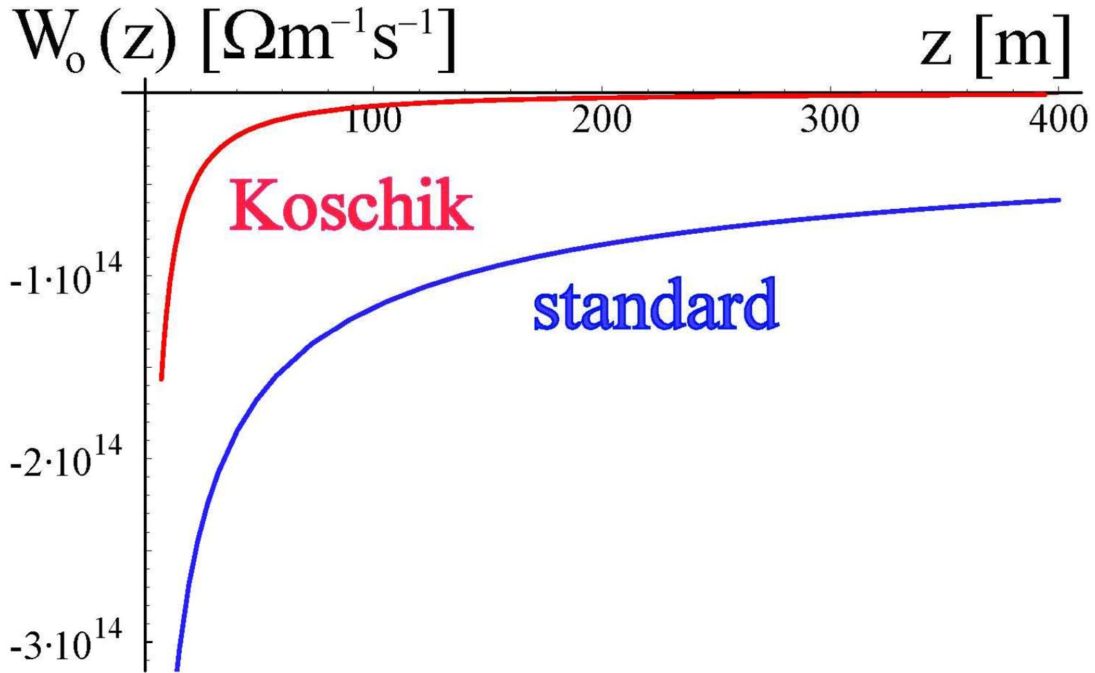
Green-function resistive-wall wake field, shown over an extended distance behind a point source, for the SPS collimator computed either from standard expression and using the Koschik formula.
