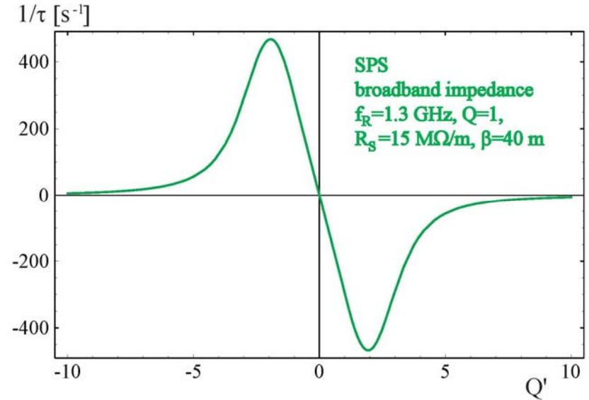
single-bunch vertical head-tail growth rates due to the SPS vertical broadband impedance.
