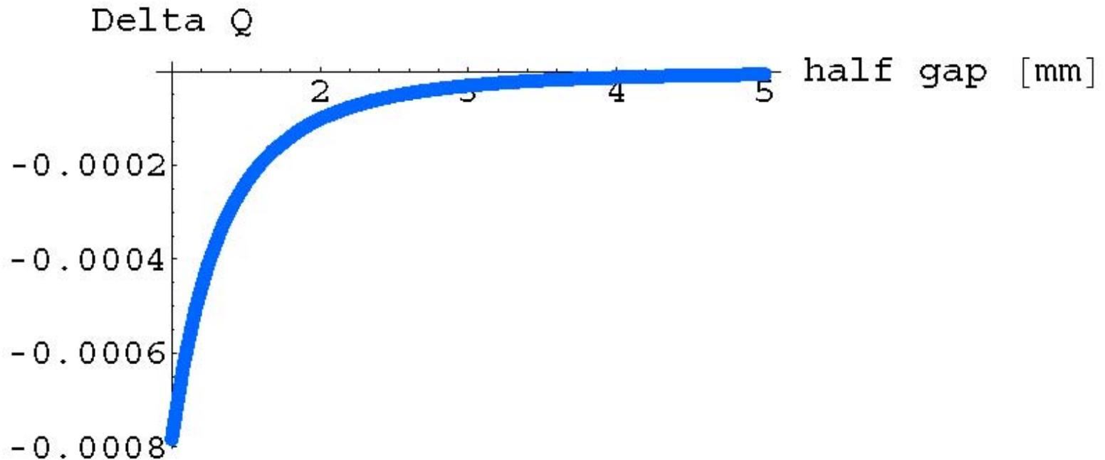
Expected tune shift versus half gap size for a pencil-like beam. Here the two jaws are closed symmetrically. Calculation assumes Burov-Lebedev resistive-wall impedance model.
