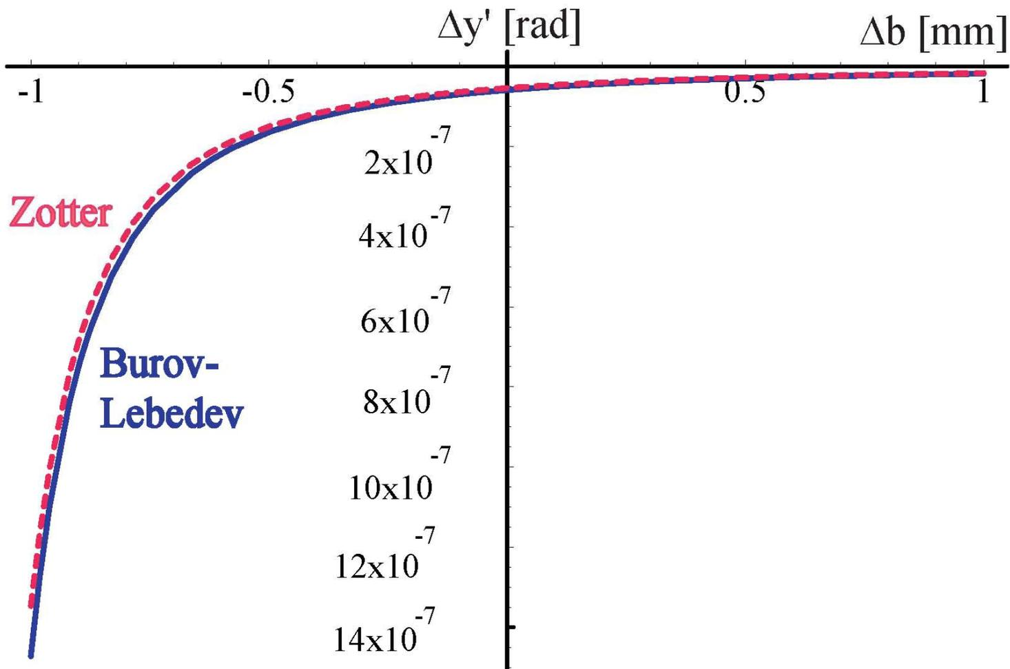
Comparison of *single-bunch deflections computed for Burov-Lebedev and Zotter impedance*. One jaw is at infinity, the other initially at 1.25 mm and then moved by an amount  $\Delta b$ . The resulting deflection of a pencil beam is shown.
