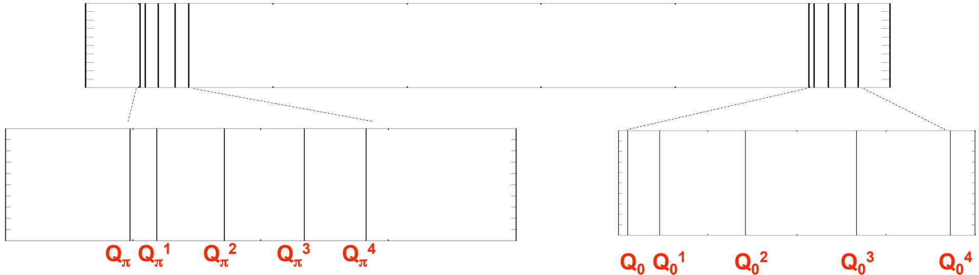
Due to the LR interaction all bunches are coupled as a result the  $\sigma$  and  $\pi$  modes split with sidebands with direction opposite with respect to the HO bb tune shift
