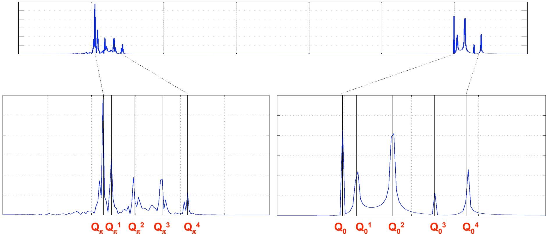
Due to the LR interaction all bunches are coupled as a result also with the **RBM** the  $\sigma$  and  $\pi$  modes split with sidebands with direction opposite with respect to the HO bb tune shift
